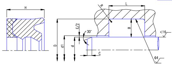
Note: 135 Series seal can be installed in open type housings to replace V-packing sets
